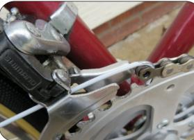
Readjusting the 'hooking' position of the tool will now allow you fit the 'Quick-link' easily without the whole lot slipping through into the grass.
