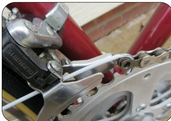
Readjusting the 'hooking' position of the tool will now allow you fit the 'Quick-link' easily without the whole lot slipping through into the grass.
